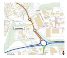
Improvements along the A388 at Carkeel by widening a section of footway and placing a new bus shelter in between the two roundabouts near Saltash Services and Tamar View Industrial Estate. The shelter will include seating, a timetable case, an advertising panel and be finished in green.
